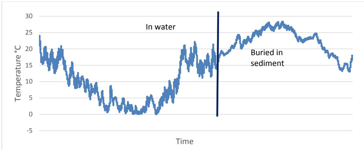
Figure 38. Example of temperature records showing a typical pattern observed when a temperature logger became buried by sediment. Daily variation decreased substantially in early May which likely indicated that the logger was buried.
