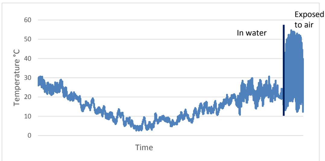
Figure 37. Example of stream temperature records showing a typical pattern observed when a temperature logger was no longer submerged. Temperature records show low variation and maximum measurements remain below 35°C while the logger was inundated followed by increased daily variability and temperatures above 45°C when the logger became exposed to the air in the late summer.
